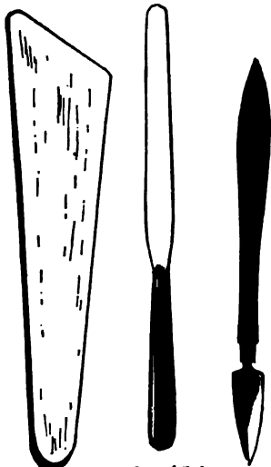
Fig. 180 Horn Palette- knife. Fig. 181 Steel Palette- knife. Fig. 182 Steel Scraper. (Reduced sizes.)
